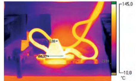
**Fig.3: Contact block and cable in visible spectrum (above) and in infrared spectrum (approx. 150 °C) (below)** (Source: W. Willand)
