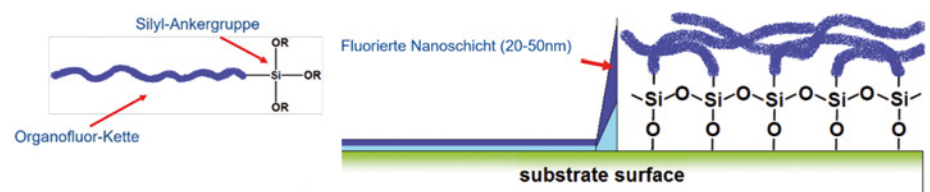
Fig. 4: Chemical structure of NanoCoat 50 and binding mechanism
