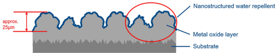
Fig. 2: Schematic layer structure of the approach
