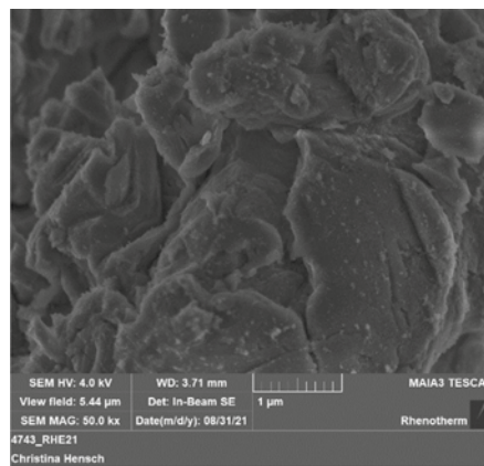
Fig. 9: SEM pictures (50,000x and 200,000x magnification) of sandblasted and hard-anodized surface with NanoCoat 50
