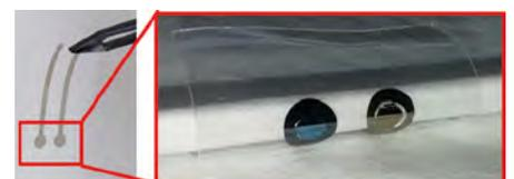
**Fig. 2: Flexible Parylene based pH sensor**
