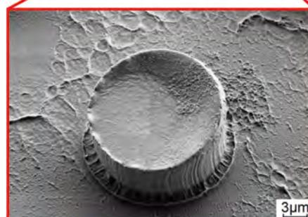
**Fig. 6: SEM image of the hot-embossed pillars on Parylene C**
