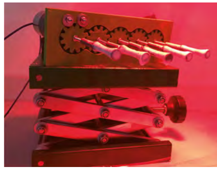
Fig. 3: Rotating moulds with liquid latex mounted on a gear drive; the moulds are placed un-
